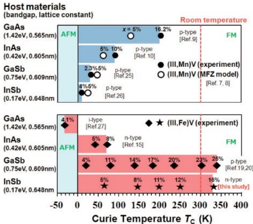
Figure 1: Highest Curie temperature ( $T_C$ ) values of Mn-doped (blue bars) and Fe-doped (red bars) III-V FMSs reported so far. The black circles, diamonds, and stars show the experimental  $T_C$  values. The white circles show the  $T_C$  values of Mn-doped III-V FMSs calculated using the mean-field Zener model. Here, AFM and FM are the antiferromagnetic and ferromagnetic couplings between the magnetic dopants, respectively.
