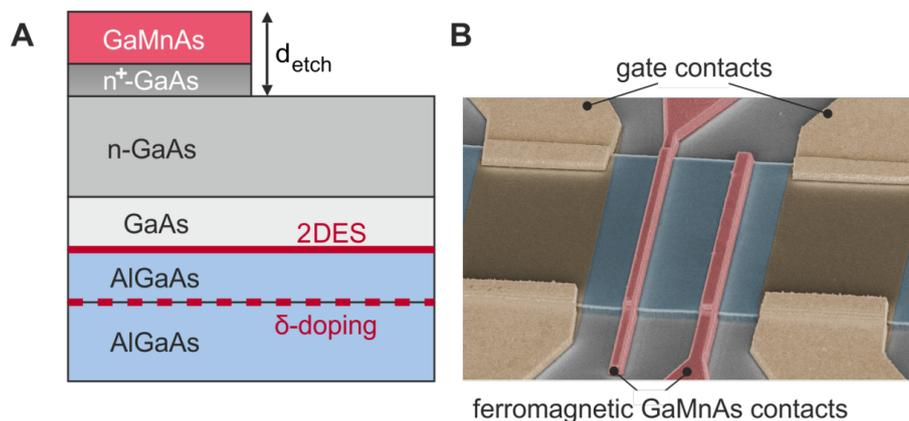
A) Layout of the heterojunctions used for spin-injection/detection. Etching of the highly doped (Ga,Mn)As and n<sup>+</sup>-GaAs layers depletes the bulk of electrons, thus enabling exclusive spin and charge transport in the 2DES. B) Device with ferromagnetic leads and gate contacts.
