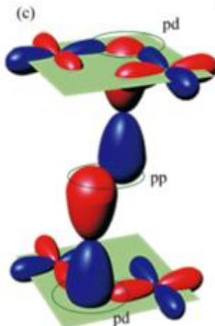
Se heights in FeSe and  $\text{FeTe}_{0.5}\text{Se}_{0.5}$  are  $1.46\text{\AA}$  and  $1.589\text{\AA}$ , shifting  $p_z$ - $d_{xy}$  down to induce a band inversion
